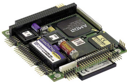
Figure 4 UAV – central processing unit (PC/104 processor module)
