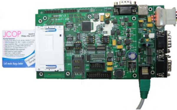
Figure 2: SCSAT04 power measurement device for cryptographic smart card analysis
