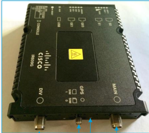
Cellular AUX GPS Cellular MAIN Dual SIM (behind SIM access cover)
